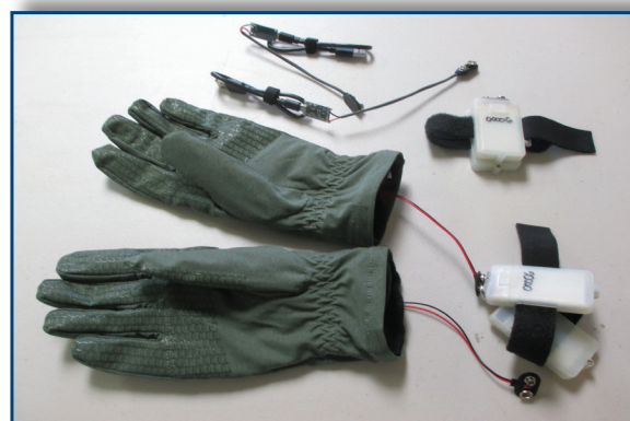
The testing prototype of Soletics heated gloves for people with Raynaud's Phenomenon.
